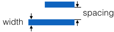
Figure 4.3 Minimum spacing and minimum width rules.
